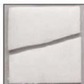
XLPE exposed 6 months in 16.5% NaOCL, 160 ft. pounds @ -40 degrees F.
